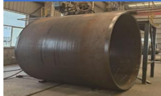
Main Leg Pipe
